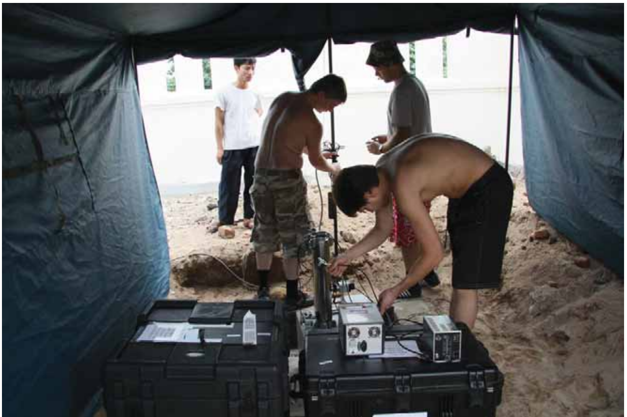
Fig.7 Absolute gravity measurement at a field gravimetric point.
