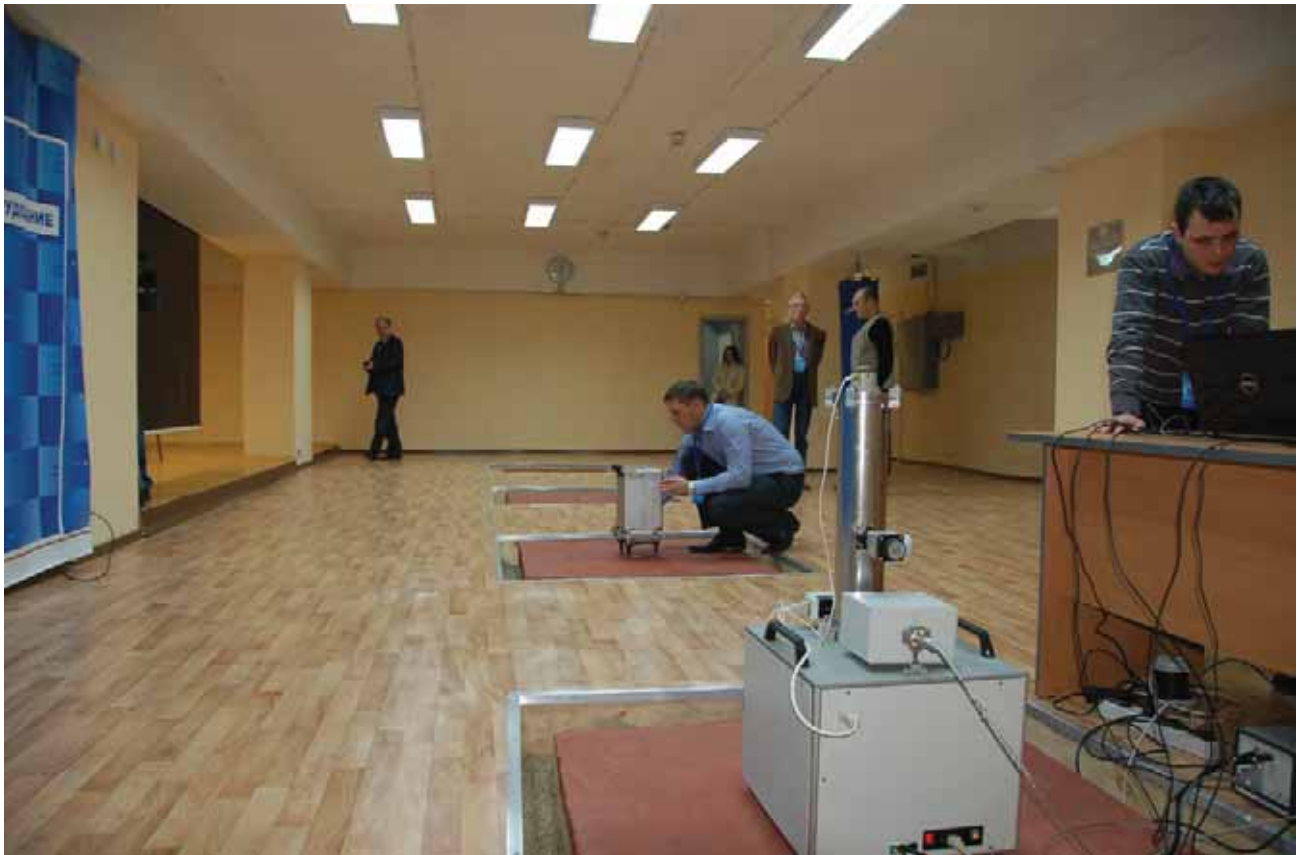
Fig. Comparison of absolute gravity meters at the site of East Siberian division of the Federal Service of Registration, Cadastre and Cartography
