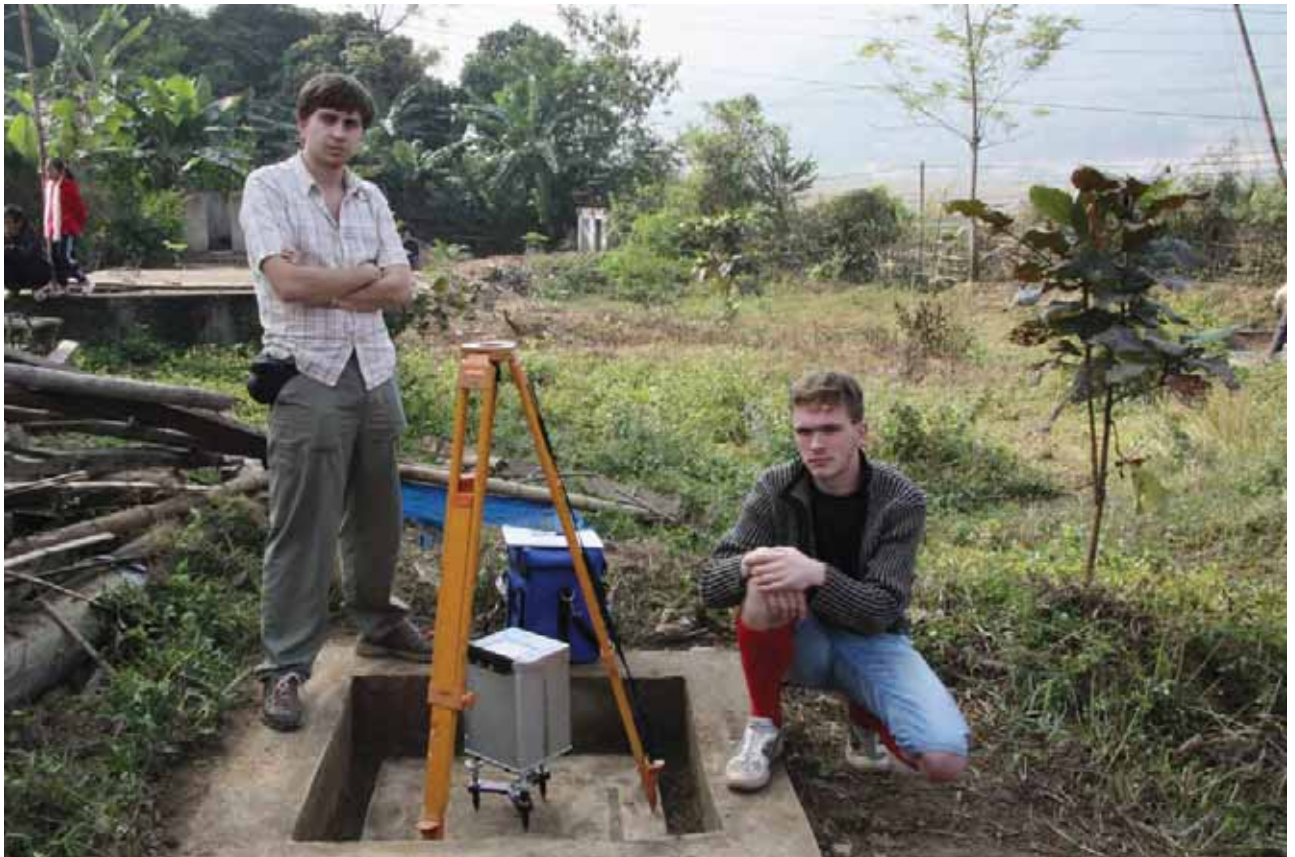
Fig.8 Relative gravity measurement at a field gravimetric point.
